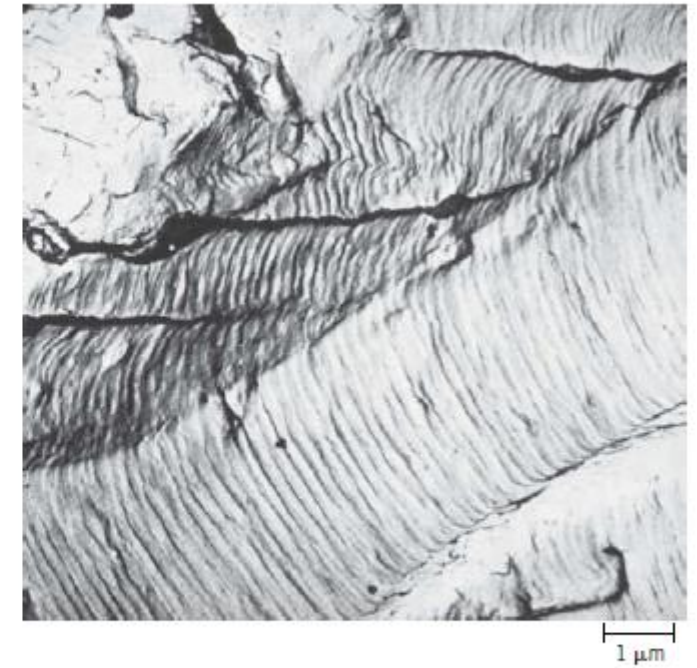
Figure 8.23 Transmission electron fractograph showing fatigue striations in aluminum. 9000 \times . (From V. J. Colangelo and F. A. Heiser, Analysis of Metallurgical Failures , 2nd edition, Copyright © 1987 by John Wiley & Sons)
