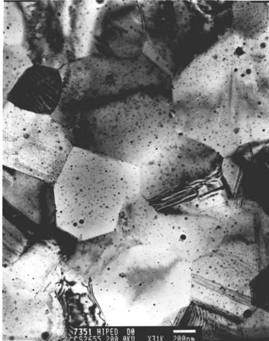
Fig. 11. Electron micrograph of the fine powder from the Ti-25Al-10Nb-3V-1Mo (at.%) + 2 wt.% Er alloy powder mechanically alloyed and HIPed. Note the uniform distribution of the \text{Er}_2\text{O}_3 dispersoids in the Ti-matrix.
