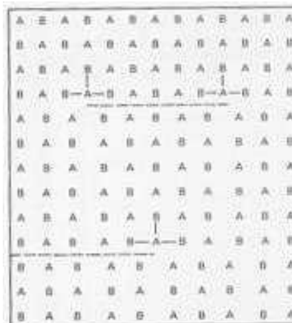
Fig. 8 Schematic representation of two types of antiphase boundaries generated by edge dislocations in an ordered alloy. The lower boundary is terminated by a single dislocation; the upper boundary, by a pair of dislocations, forming a superlattice dislocation.
