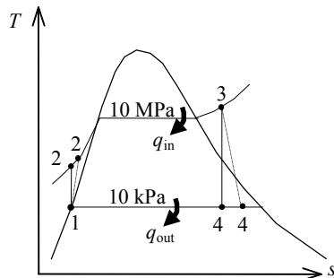
**10-20** A 300-MW coal-fired steam power plant operates on a simple ideal Rankine cycle between the specified pressure limits. The overall plant efficiency and the required rate of the coal supply are to be determined.
