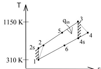
**9-98** A regenerative gas-turbine engine using air as the working fluid is considered. The amount of heat transfer in the regenerator and the thermal efficiency are to be determined.
