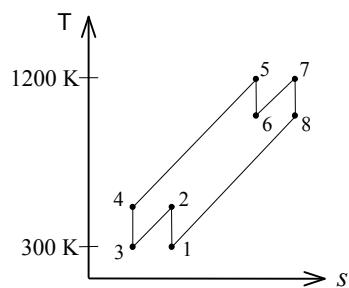
**9-111** A regenerative gas-turbine cycle with two stages of compression and two stages of expansion is considered. The minimum mass flow rate of air needed to develop a specified net power output is to be determined.
