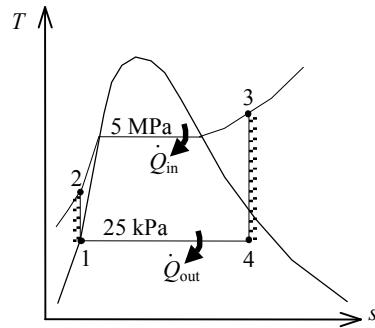
**10-22** A steam power plant operates on a simple ideal Rankine cycle between the specified pressure limits. The thermal efficiency of the cycle, the mass flow rate of the steam, and the temperature rise of the cooling water are to be determined.
