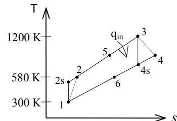
**9-110** A regenerative gas-turbine cycle with two stages of compression and two stages of expansion is considered. The minimum mass flow rate of air needed to develop a specified net power output is to be determined.
