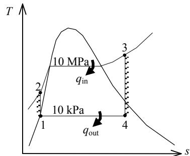
**10-17** A steam power plant that operates on a simple nonideal Rankine cycle is considered. The quality of the steam at the turbine exit, the thermal efficiency of the cycle, and the mass flow rate of the steam are to be determined.
