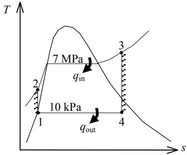
**10-23** A steam power plant operates on a simple nonideal Rankine cycle between the specified pressure limits. The thermal efficiency of the cycle, the mass flow rate of the steam, and the temperature rise of the cooling water are to be determined.
