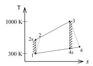
9-77 A stationary gas-turbine power plant operates on a simple ideal Brayton cycle with air as the working fluid. The power delivered by this plant is to be determined assuming constant and variable specific heats.
