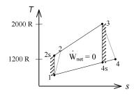
$$\dot{Q}_{\text{out}} = \dot{m}(h_4 - h_1) \longrightarrow h_1 = 291.30 - 6400/40 = 131.30 \text{ Btu/lbm} \longrightarrow P_{r_1} = 1.474$$
