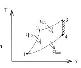
**9-19** The three processes of an air-standard cycle are described. The cycle is to be shown on P-v and T-s diagrams, and the heat rejected and the thermal efficiency are to be determined.
