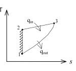
**9-20** The three processes of an air-standard cycle are described. The cycle is to be shown on P-v and T-s diagrams, and the net work per cycle and the thermal efficiency are to be determined.
