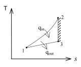
**9-21** The three processes of an air-standard cycle are described. The cycle is to be shown on P-v and T-s diagrams, and the net work per cycle and the thermal efficiency are to be determined.
