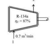
$$\eta_c = \frac{h_{2s} - h_1}{h_{2a} - h_1} \longrightarrow h_{2a} = h_1 + (h_{2s} - h_1)/\eta_c = 234.44 + (282.51 - 234.44)/0.87 = 289.69 \text{ kJ/kg}$$
