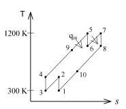
Thus,  $r_{\text{bw}} = \frac{w_{\text{C,in}}}{w_{\text{T,out}}} = \frac{222.14 \text{ kJ/kg}}{662.86 \text{ kJ/kg}} = 33.5\%$   $q_{\text{in}} = (h_5 - h_4) + (h_7 - h_6) = (1277.79 - 411.26) + (1277.79 - 946.36) = 1197.96 \text{ kJ/kg}$   $w_{\text{net}} = w_{\text{T,out}} - w_{\text{C,in}} = 662.86 - 222.14 = 440.72 \text{ kJ/kg}$   $\eta_{\text{th}} = \frac{w_{\text{net}}}{q_{\text{in}}} = \frac{440.72 \text{ kJ/kg}}{1197.96 \text{ kJ/kg}} = 36.8\%$
