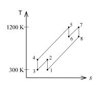
**9-111** A regenerative gas-turbine cycle with two stages of compression and two stages of expansion is considered. The minimum mass flow rate of air needed to develop a specified net power output is to be determined.
