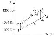
$$\begin{split} P_{r_4} &= \frac{P_4}{P_3} \, P_{r_3} = \left(\frac{1}{8}\right) (238.0) = 29.75 \longrightarrow h_{4s} = 719.75 \text{ kJ/kg} \\ \eta_T &= \frac{h_3 - h_4}{h_3 - h_{4s}} \longrightarrow h_4 = h_3 - \eta_T \left(h_3 - h_{4s}\right) \\ &= 1277.79 - \left(0.86\right) (1277.79 - 719.75) \\ &= 797.88 \text{ kJ/kg} \end{split}$$
