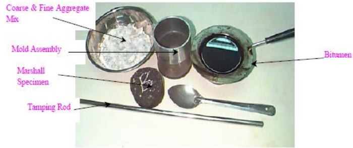
Figure 11.3 Test Specimen Preparation
