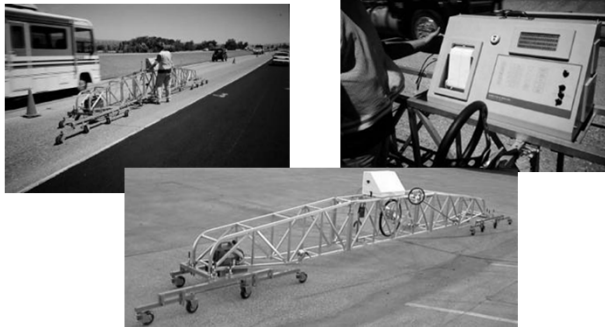
Truss-type profilograph and output data
