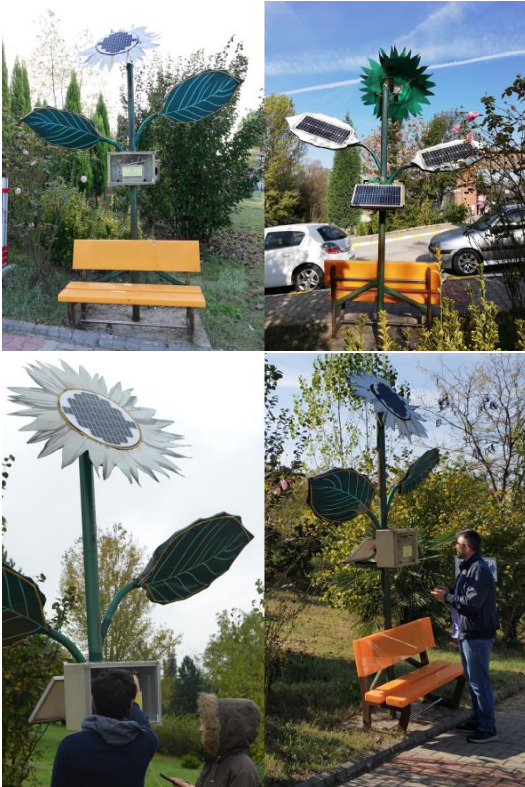
Solar energy system for charging devices like telephone etc.
